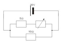
The resistance of the variable resistor is gradually increased from zero to 5  $\boldsymbol{\Omega}.$
