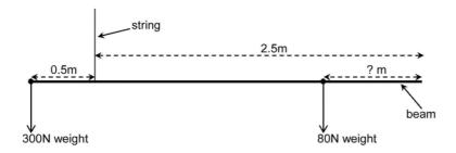
How far from the other end must a weight of 80N be placed for the beam to be balanced?
