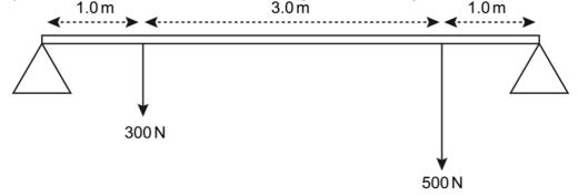
What are the upward forces from the two supports acting on the beam?
