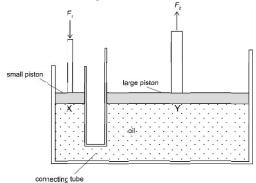
A downward force  $F_1$  is applied to the smaller piston, which results in an upwards resultant force  $F_2$  being exerted on the larger piston. Points X and Y are in the oil, immediately underneath the pistons, which are at the same height.
