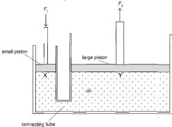
A downward force  $F_1$  is applied to the smaller piston, which results in an upwards resultant force  $F_2$  being exerted on the larger piston. Points X and Y are in the oil, immediately underneath the pistons, which are at the same height.
